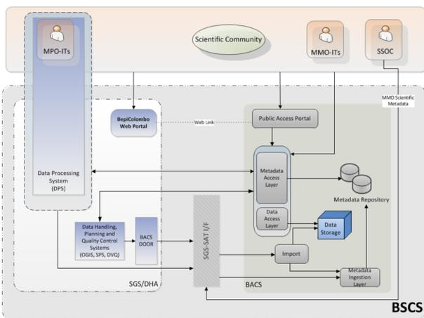
The role of the BACS as a subsystem of the BSCS is to act as a central distribution system and to facilitate the information exchange of data and metadata between the core subsystems of the BSCS as well as with the MPO Instrument Teams.
