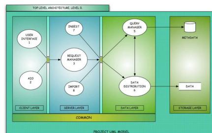
The BACS builds on top of the SAT's common Archives Building System Infrastructure (ABSI), which defines the components common to all the current ESA Science Archives within a three-tier modular architecture.
